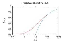
But frictional drag halves the Propulsion at low Re.
