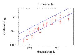
Grooves 5 heights & 4 lengths, Plates 3 thickness, ( $K = 0.15 \rightarrow 2800, Re = 1 \rightarrow 200$ )  $a = 0.02 \rightarrow 1.4 \,\mathrm{m/s^2}$
