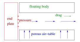
End plate attached to base (grooved table)  $\longrightarrow$  body dragged by flow to right End plate attached to top (grooved body)  $\longrightarrow$  pressure pushes to left
