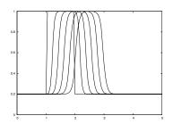
$ct=0.0\,(0.2)\,1.0$   $\Delta x=0.05$  and  $c\Delta t=0.0125$  slightly sharper than Minmod
