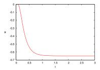
Steady to  $10^{-4}$  by t = 2, time to diffuse across box. For steady state, try reducing to 3 SOR per time step in place of *N*.
