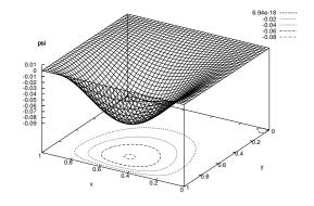
Fast near lid, slow deep into cavity. Weak reversed circulations in bottom corners At t = 3, Re = 10 and N = 40.
