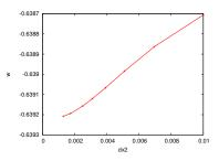
Linear in  $\Delta x^2$ . Result:  $\omega(0.5, 0.5, 1) = -0.63925 \pm 0.00005$ . Note linear extrapolation in  $\Delta x^2$  from N = 10 and 14 gives same accuracy as 28 at  $\frac{1}{32}$  the CPU.
