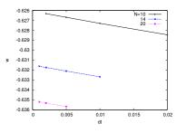
Note: linear in  $\Delta t$ , very very small  $\Delta t$  (larger unstable), Large errors in  $\Delta x \rightarrow 2$ nd order BC for  $\omega_0$  better?
