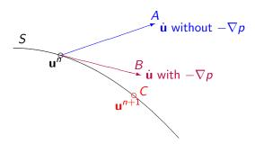
Avoid slow accumulation of errors by projecting  ${\bf u}$  back onto surface at  ${\bf C}$
