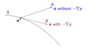
Role of  $\nabla p$  is to project out component of  $\partial \mathbf{u}/\partial t$  normal to surface.
