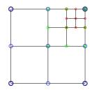
Time-step stability controlled by smallest grid block
