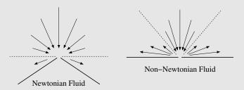
Rigid-rod suspension, with the compression in  $\theta\text{-direction},$  has recirculation region at angle  $=\pi$
