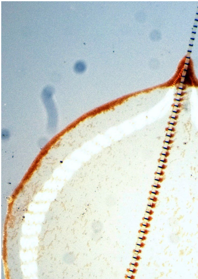
Figure 2. Collective transport of magnetic microparticles on an artificial microtubule near a droplet.
