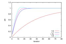
For N = 20 Gauss-Seidel needs 500 iterations, whereas SOR with optimal  $r \approx 1.75$  needs 20.
